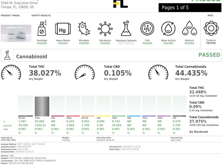
Full Spectrum cannabinoid analysis utilizing High Performance Liquid Chromatography with UV detection in accordance with F.S. Rule 64ER20-39
