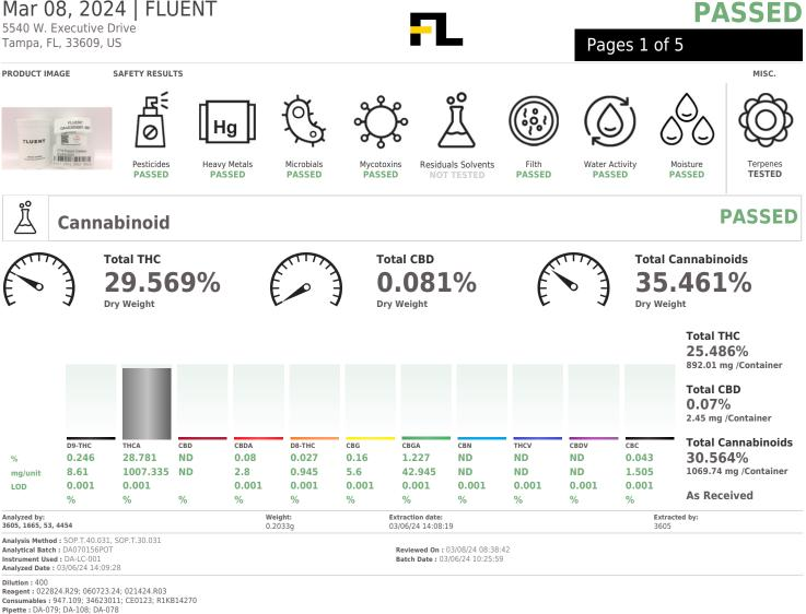
Full Spectrum cannabinoid analysis utilizing High Performance Liquid Chromatography with UV detection in accordance with F.S. Rule 64ER20-39
