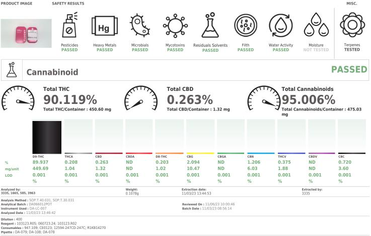
Full Spectrum cannabinoid analysis utilizing High Performance Liquid Chromatography with UV detection in accordance with F.S. Rule 64ER20-39
