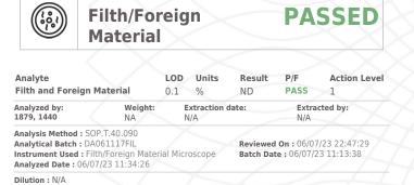
Filth and foreign material inspection is performed by visual inspection utilizing naked eye and microscope technologies in accordance with F.S. Rule 64ER20-39.
