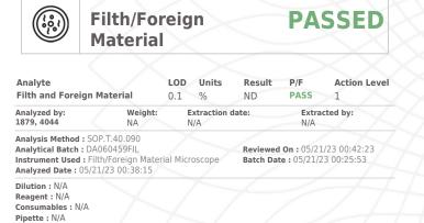
Filth and foreign material inspection is performed by visual inspection utilizing naked eye and microscope technologies in accordance with F.S. Rule 64ER20-39.
